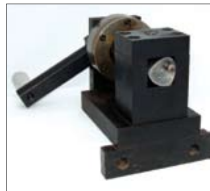
This device, based on a variation of the Reuleaux triangle, drills holes that are perfectly square. From How Round Is Your Circle?
