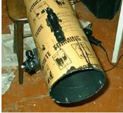
Figure 11: Telescope with focuser (left) and finder (right). Note that the telescope is tilted, the finder is not actually directly on the top of the tube.
