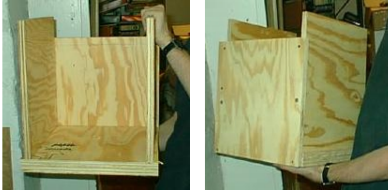
Figure 10: Views of the rocker box, from front and back
