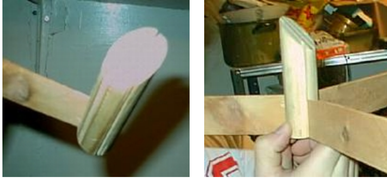
Figure 4: The spider with one fin (left) and all fins (right) attached
