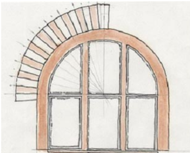
Decorative Brickwork frames windows.
